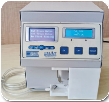
Advance version of Electronic Milk Adulteration Tester (EMAT+)
